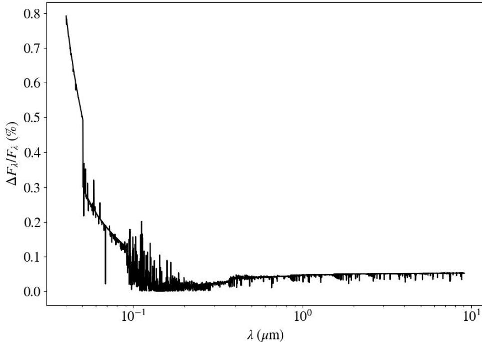
The relative radiative flux difference between a plane-parallel and a spherical model is below 0.1 % in the wavelength interval we use. We, thus, have done all the calculations with the plane-parallel geometry to reduce the computing time
