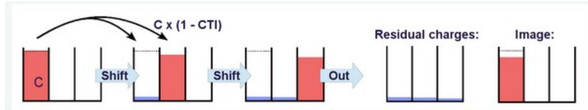
Electrons captured by traps (during the charge transfers) and released after a while:
