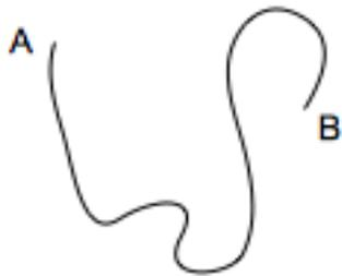
$$\int_C \vec{E} \cdot d\vec{\ell} = \int_C -\text{grad}V \cdot d\vec{\ell} = - \int_A^B dV = V(A) - V(B)$$
